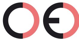
False CE Mark (too far)
